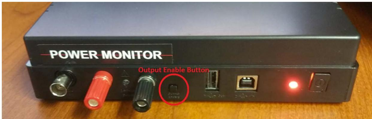
**Figure 3** Output Enable button
