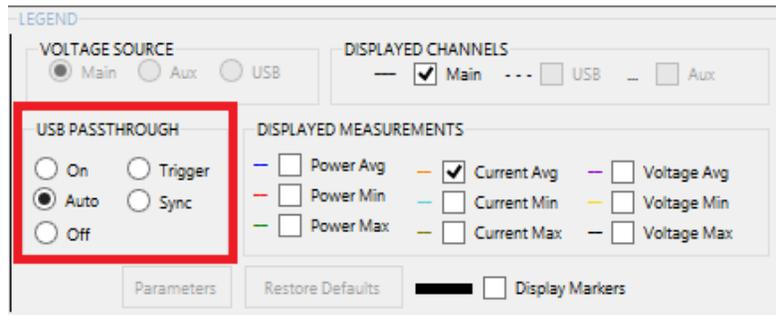
**Figure 29** USB pass-through control
