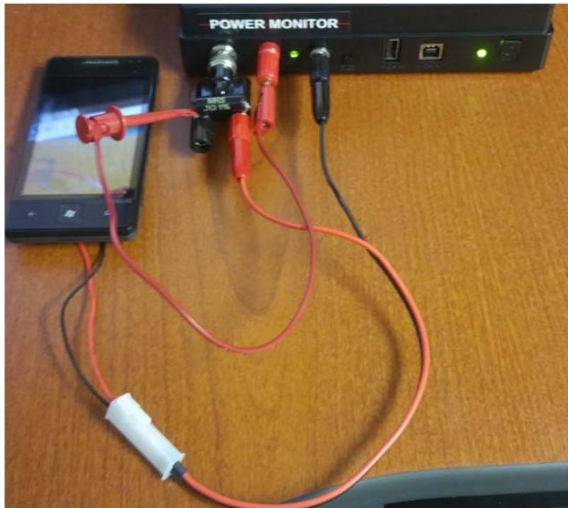
**Figure 37** Example connection to the Aux port
