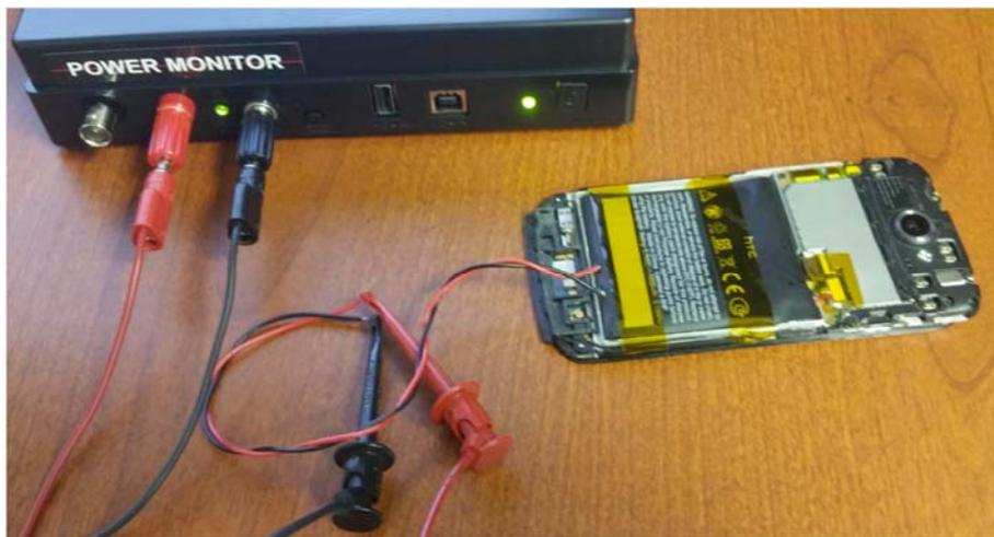
**Figure 8** A mobile device connected to the main channel
