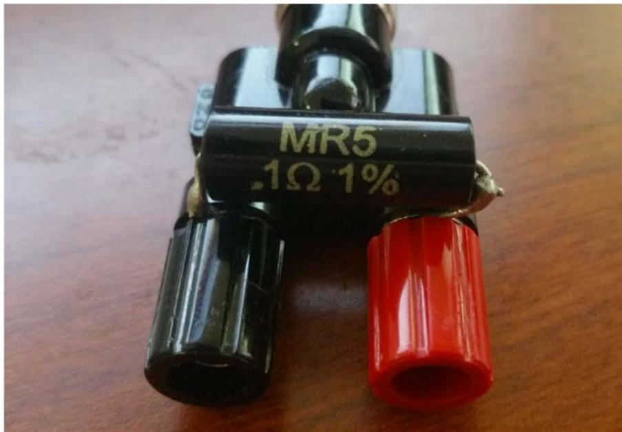
**Figure 33** 0.1 ohm sense resistor
