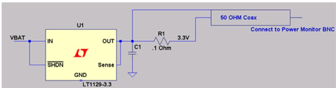
**Figure 36** Schematic of the Aux port connection
