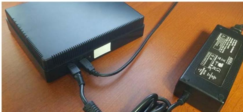
**Figure 6** Back view: Power connector and USB connector
