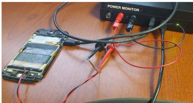
**Figure 28** USB device connection, including main channel connection
